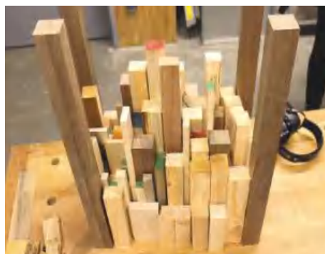
▲ Pic.2 To get an idea of placement, assemble your table upside down
